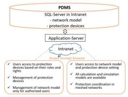
Using a sophisticated user administration scheme, PDMS offers different types of accessibility to the master database that contains the complete network model and all protection devices. Intranet users have direct access to PDMS database. Desktop users store their project in a local database with bidirectional communication with the PDMS database.
