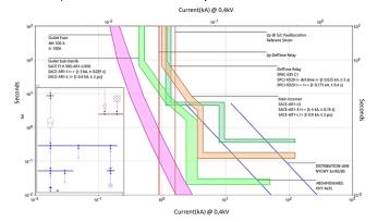
NEPLAN offers easy interaction between the singleline diagram and the selectivity chart which is automatically generated after a short circuit calculation.
